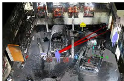
I-Site Forensic™ provides investigators with the tools needed to record scene evidence and points of interest and create an extremely accurate 3D virtual representation of this information for communicating and analysing after the fact.
